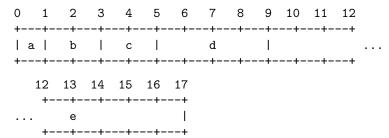
With an alignment of 2, the struct members larger than one byte would be aligned to 2-byte boundaries, which results in a single padding byte between a and b.
