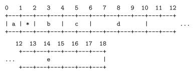
With an alignment of 4, the struct members of size 2 would be aligned to 2-byte boundaries and larger struct members would be aligned to 4-byte boundaries:
